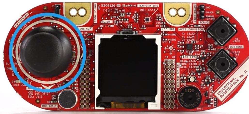
**Figure 5. 2-Axis Analog Joystick With Digital Input**
