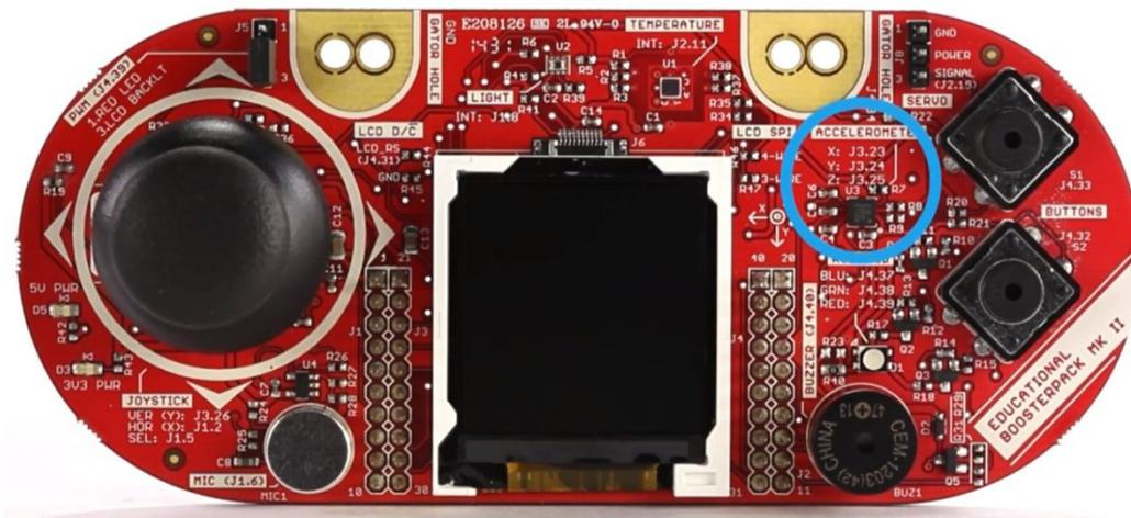
**Figure 4. 3-Axis Analog Accelerometer**
